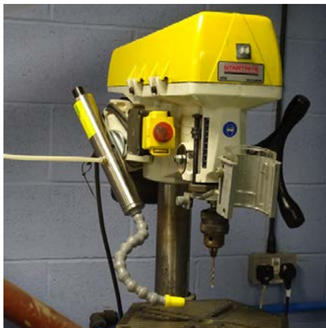
Adjustable Coldstream Air Gun used to cool drill.
