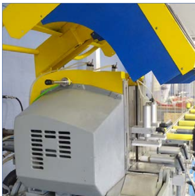
Vortex Tube used to cool saw blade.
